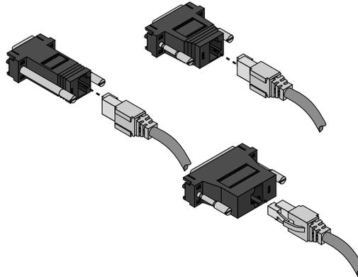
2. Connect the interface adapter in any of the remaining serial ports labeled **2-8**. Serial port **1** is reserved for the monitor.
