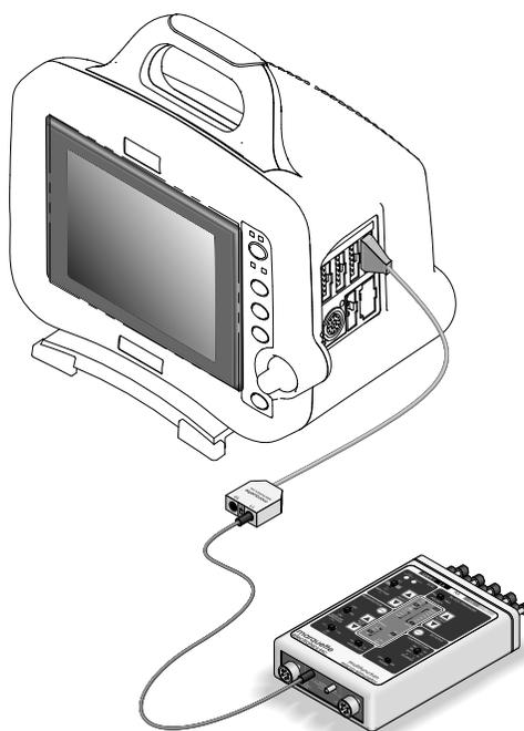
2. Turn on the simulator, set the adapter to 400 and set the temperature output to 37°C.
