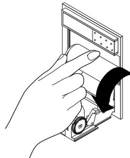
2. Remove the old spool and install a new paper roll. Install the paper so it unrolls from the bottom.
